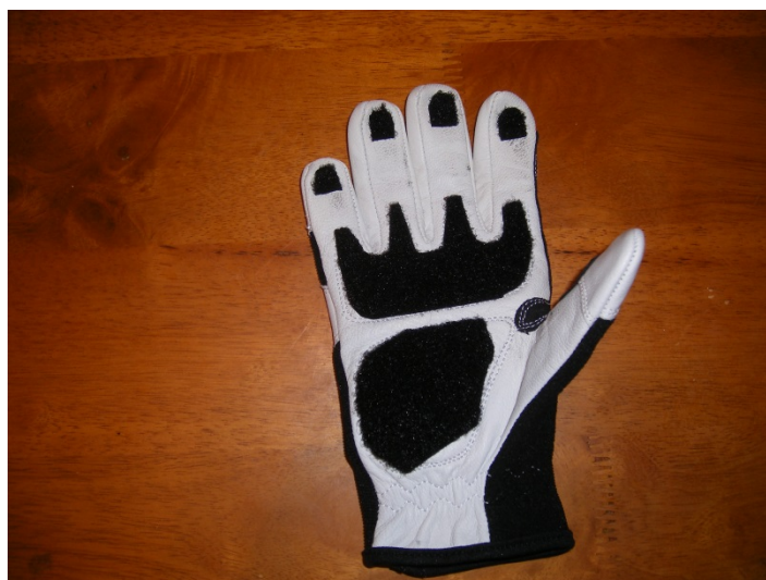
Figure 3—Previous attempt, with Velcro on the palmar side of the glove
